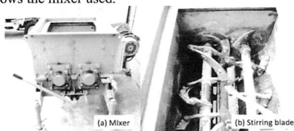
Figure 1. A photograph of a mixer for test production of the Anti-Sievert® concrete.
